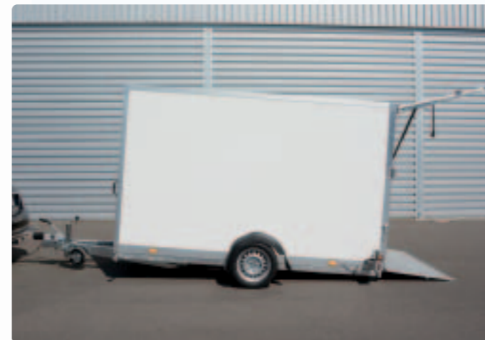
AZSL 1730/176 Heckrampe aus Aluprofilen, Sandwichpolyesterheckklappe AZSL 1730/176 Pont arrière en profilés d'aluminium, clapet en polyester sandwich AZSL 1730/176 Rear ramp made of alum. profiles, sandwich polyester hatch
